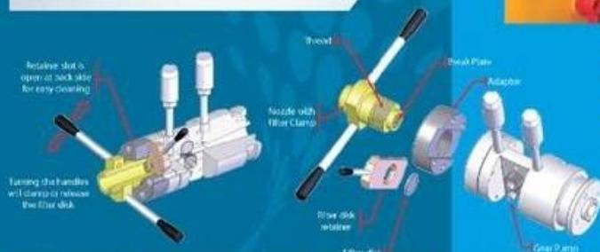
Our filter test head with gear pump is designed specifically for easy cleaning where the melt flows in a straight line from extruder through gear pump all the way up to the filter. The filter is easily installed and removed with our quick clamping system.
